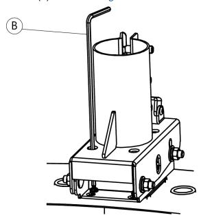
Figure 46: Tightening the blind mate guide screws
