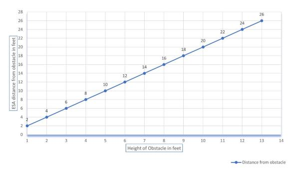
Figure 3: Distance of ESA from obstacle
