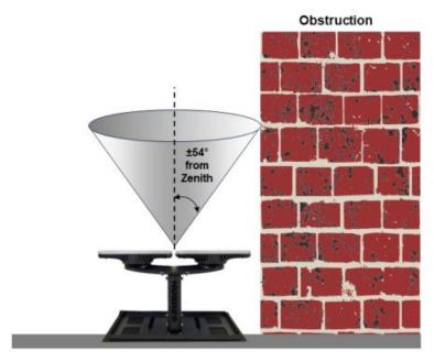
Figure 4: Incorrect placement of ESA, with clear blockage of the conical view
