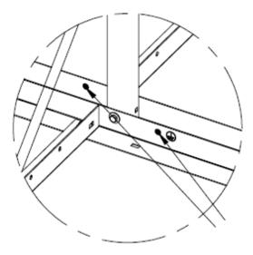
Figure 37: Tearing off the grounding stickers
