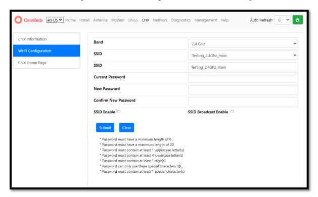
Figure 139: ODU LUI Wi-Fi Configuration screen
