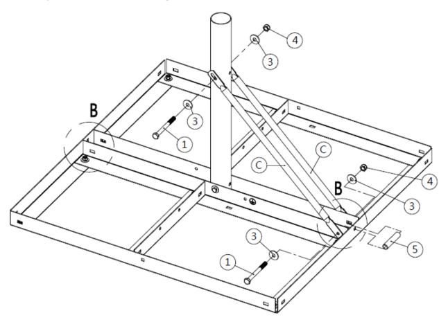
Figure 35: Installing the first two side supporting rods
