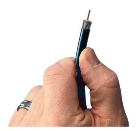
Figure 61: Exposing the braid and foil
