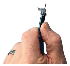
Figure 63: Cutting the inner foil
