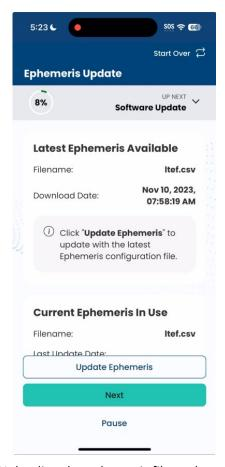
Figure 96: Uploading the ephemeris file to the user terminal
