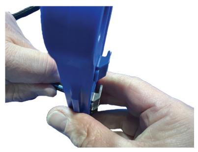
Figure 58: Pulling the cable from the strip tool
