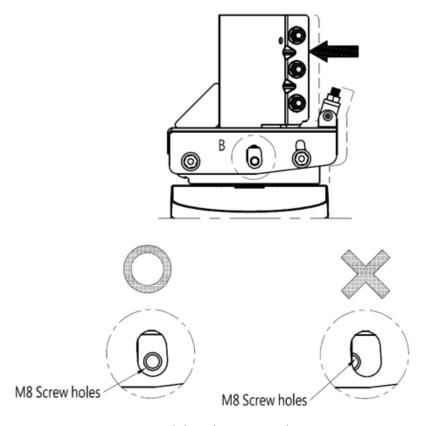
Figure 43: Sliding the mount adapter
