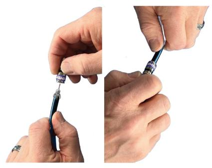
Figure 65: Inserting the IFL cable into the connector
