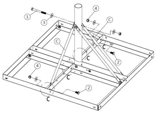
Figure 36: Installing the second two side supporting rods
