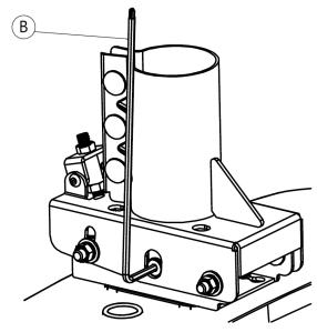
Figure 45: Tightening the mount adapter side screws
