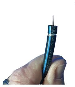
Figure 60: Exposing the center conductor
