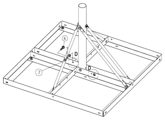
Figure 38: Installing the grounding cable
