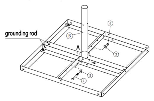
Figure 33: Installing the mast pole
