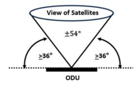
Figure 2: ODU operational conical view of Satellites
