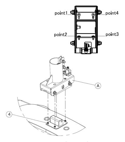
Figure 42: Mounting the mount adapter
