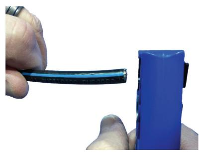
Figure 56: Inserting the IFL cable into the strip tool
