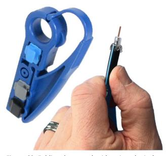
Figure 62: Folding the outer braid against the jacket
