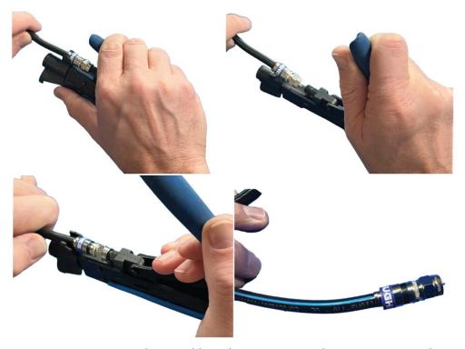
Figure 66: Inserting the IFL cable and connector into the compression tool
