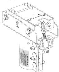
Figure 41: Installing the radiation hazard caution label
