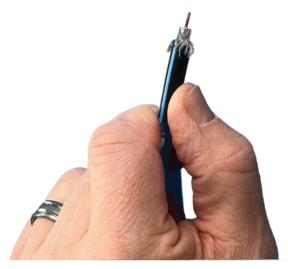
Figure 64: Folding the inner braid against the folded outer braid
