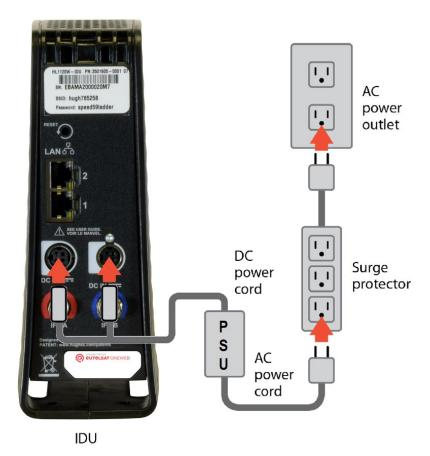
Figure 70: IDU power diagram
