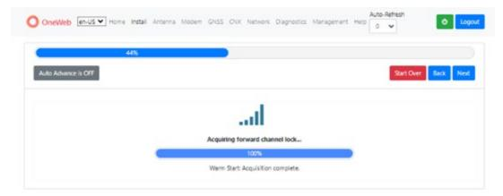
Figure 125: LUI – Forward channel lock screen
