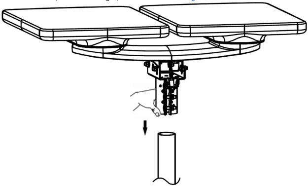
Figure 47: Mounting the ODU onto the mast pole
