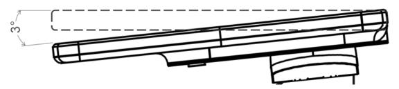
Figure 22: Tilting the ODU forward to 3-degrees
