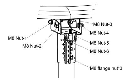
Figure 49: Tightening azimuth and tilt screws
