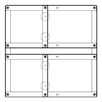
Figure 39: Penetrating fastener mount locations
