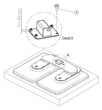
Figure 40: Installing the blind mate guide
