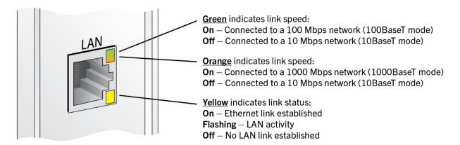
Figure 147: LAN port LEDs
