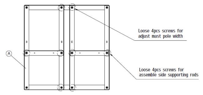
Figure 32: Loosening the ground mounting screws
