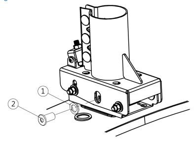
Figure 44: Installing the mount adapter side screws
