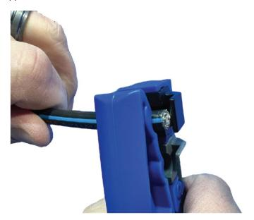
Figure 57: Rotating the cable strip tool
