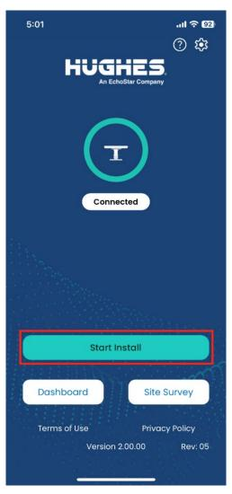
Figure 86: Start Install button to start fresh commissioning
