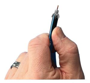
Figure 60: Folding the inner braid against the folded outer braid
