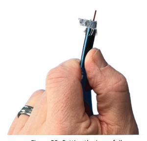
Figure 59: Cutting the inner foil
