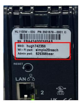
Figure 67: HL1100W-IDU Wi-Fi SSID and Passwords
