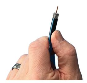
Figure 57: Exposing the braid and foil
