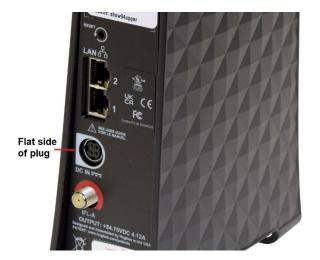
Figure 65: Proper power cord orientation
