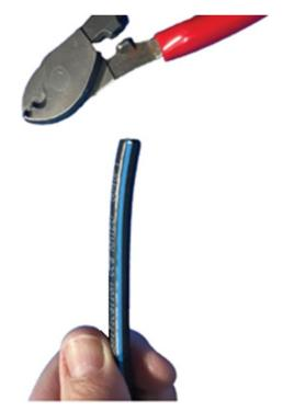
Figure 51: Cutting the IFL cable to length
