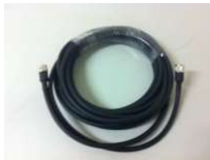
Figure 2: RF cable with N to TNC adapter P/N 3500634-0001
