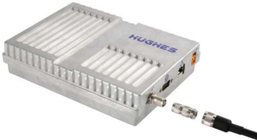
Figure 31: Connect cable to TNC connector on IDU
