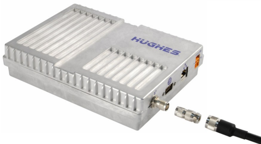
Figure 32: Connect cable to TNC connector on IDU
