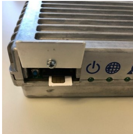
Figure 33: Installing the SIM card
