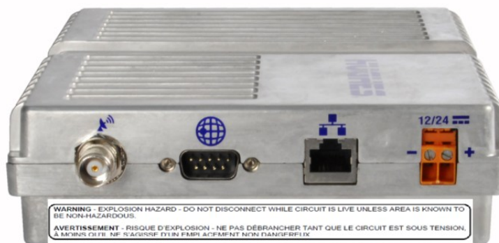
Figure 8: Back side view of IDU
