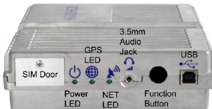
Figure 7: Front side view of IDU
