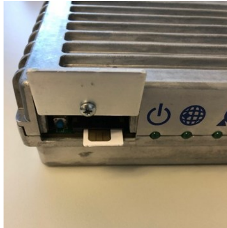
Figure 33: Installing the SIM card
