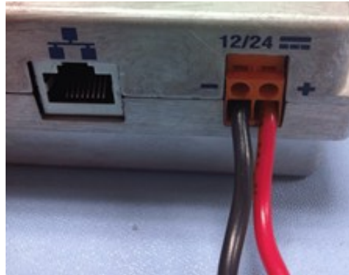
Figure 35: Connecting power leads
