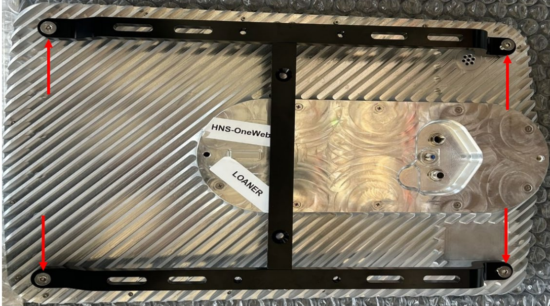
Figure 11: Securing the mount to the HL1100
