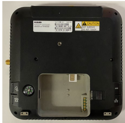
Installing the USIM
