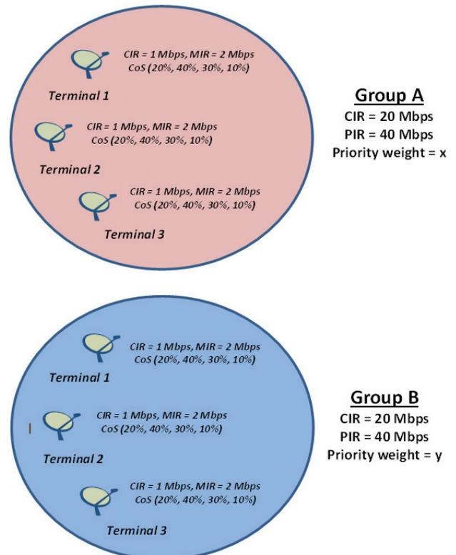
The JUPITER System ensures maximum efficiency in bandwidth utilization. The combination of QoS and bandwidth management techniques ensures applications are prioritized accordingly.
