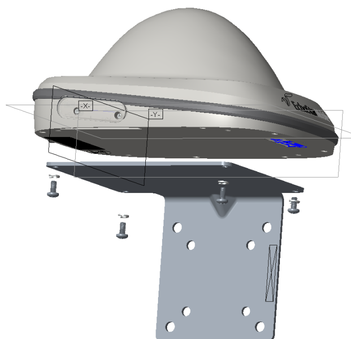
Figure 9: Placing the plate and tightening the screws
