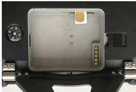
3. Install the battery and completely charge it with the AC/DC adapter before using the terminal.
