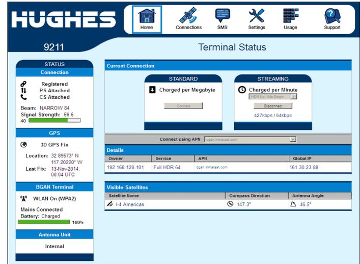
10. Press the “Register with network” button. The UT will register and attach to the Inmarsat network.
