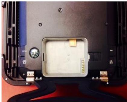
3. Install the battery and completely charge it before using the terminal.
