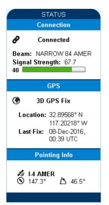
The status bar is included on the home page and other pages that do not have a navigation bar. It includes a field with the elevation angle and compass direction towards the visible satellite(s).
