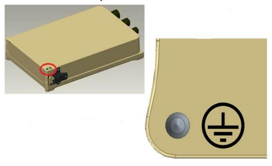
Figure 5-1 – LPB Protective Earth Grounding
