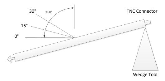
Figure 4-8: 0° to 30° Elevation Angle
