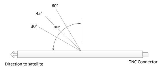
Figure 4-7: Typical Lay Flat Antenna Pointing 30° - 60° Elevation Angle
