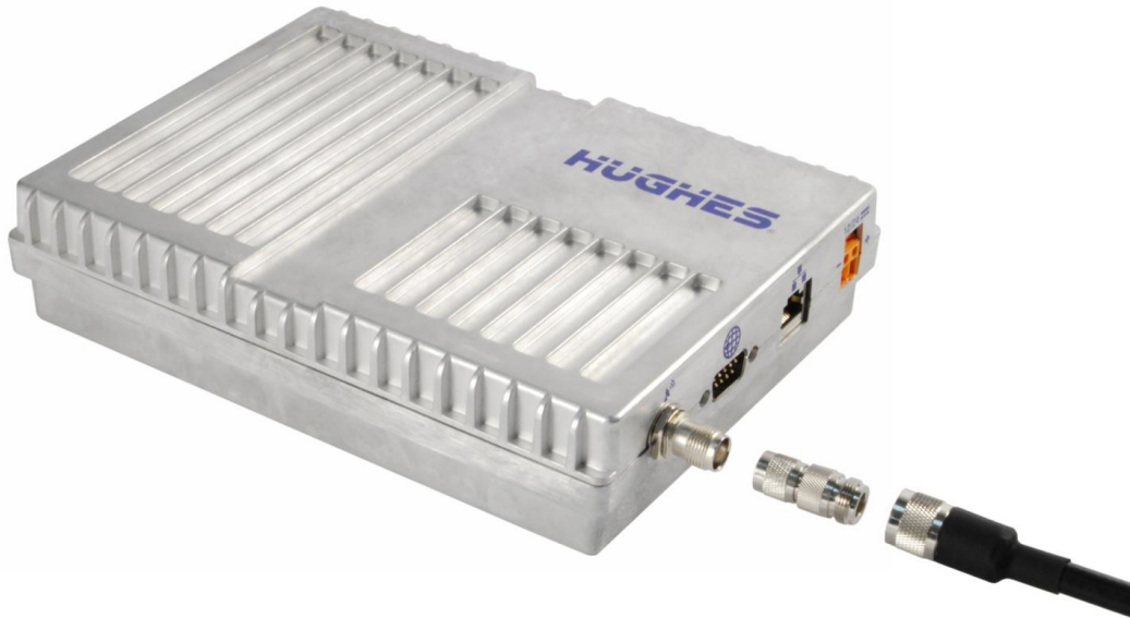
Figure 34: Connect cable to TNC connector on IDU
