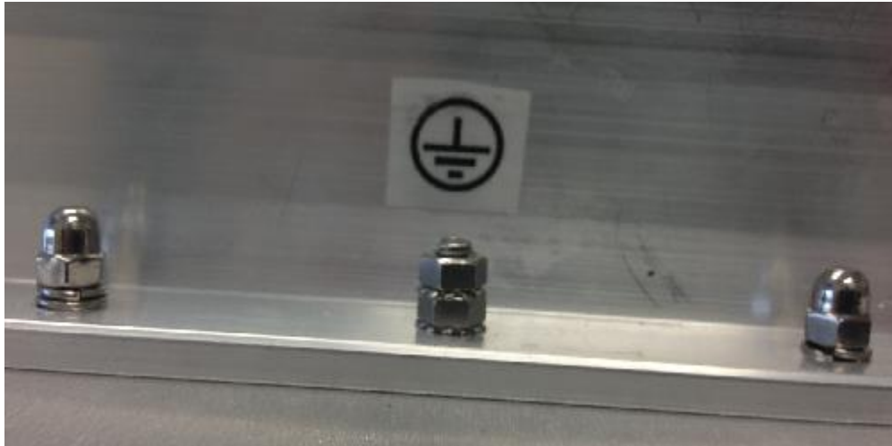
Figure 47: 9502 Protective earth grounding
