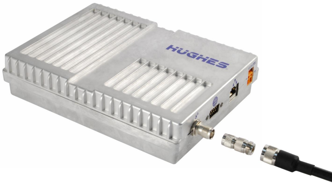
Figure 32: Connect cable to TNC connector on IDU
