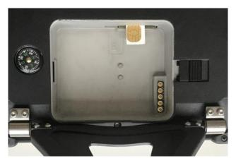
Figure 2: Inserting the USIM card
