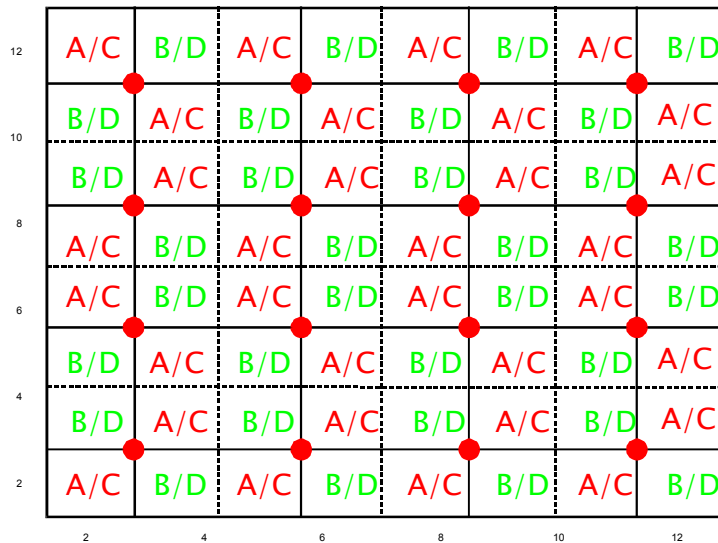
Figure 8-1. Frequency Plan with 90° Sector, Two-Channel Reuse
