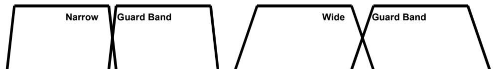
Figure 6-4 Narrow and Wide Guard Bands (The width of the guard band is a function of many design and engineering factors. All things being equal, for a given channel spacing the system with the narrower guard band will have a greater throughput.)
